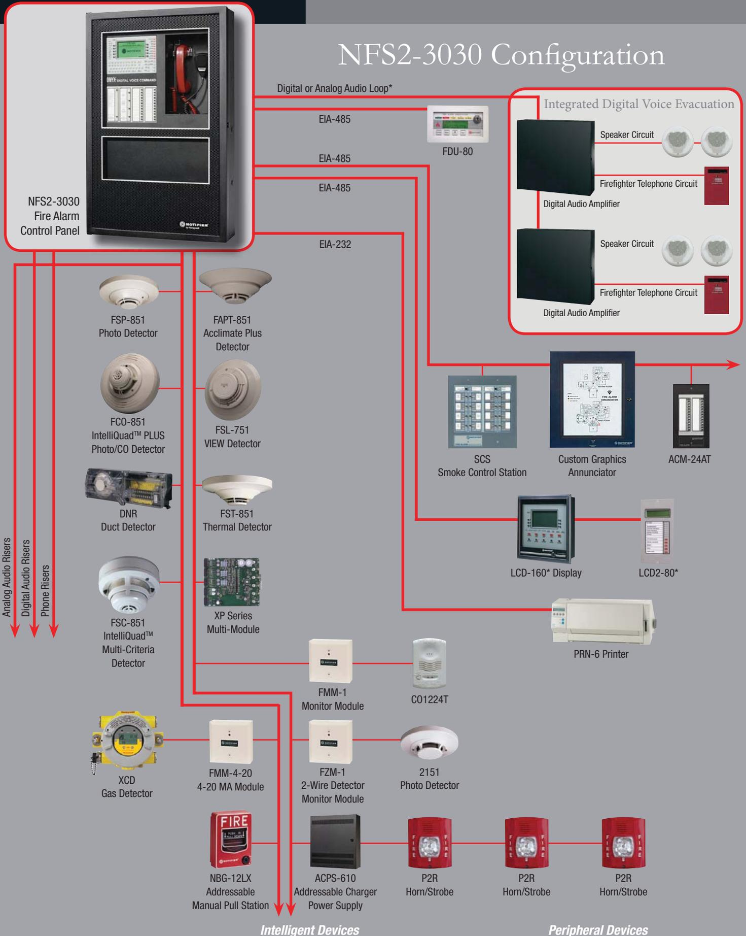
\*RDP port can support LCD-160 or LCD2-80 in Terminal Mode, but not at the same time.
